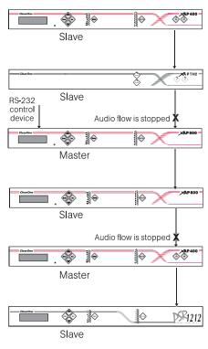
Figure 2.5. E-bus network with master units
